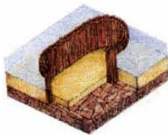
Fig. 1.3 – Cofferdam for foundation
